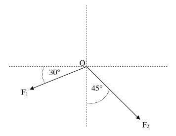
If  $|F_1| = 1600$  N and  $|F_2| = 900$  N, determine the magnitude and bearing of a single force  $F_3$  that would keep the system in equilibrium.
